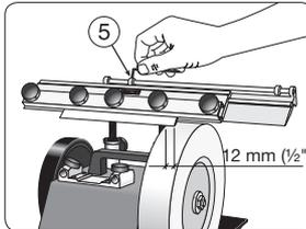
Place the blade holder on the support. Set the grinding length to the length of the blade to ensure that the blade does not run off the edge of the stone during grinding. This is done by adjusting and locking both stops (5). Blades longer than approx 270 mm (10 1/2"), you move in the holder and grind in two steps.\*
