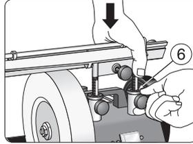
Press down the grinding jig while locking with the locking screws so that the two wheels (6) rest on the base without any gap.
