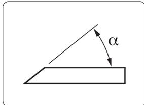
Grind the blade at exactly the original edge angle ( $\alpha$ ).
