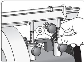
Make an initial height setting with the wheels (6). Set the edge angle with the adjusting screw (7). Make fine adjustments to the height with the wheels (6). The bevel should now lie flat on the stone and the holder (2) should touch the support (1).
