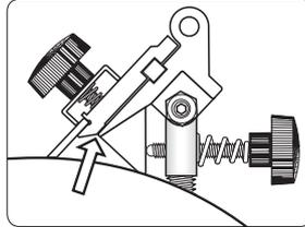
You must grind until the blade holder rests against the support along the whole length. Grind the other blade with the same setting.
