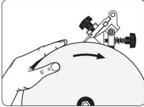
Check the angle setting by turning the wheel by hand. The wheel should make marks on the whole bevel, from the tip to the heel.
