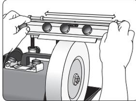
Grind by moving the holder with even pressure from side to side between the side stops.
