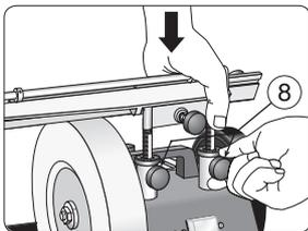
Lock the support plate – while it is pressed down – with the two locking screws (8).
