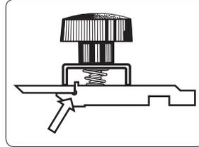
Clamp the blade in the holder. Make sure that it rests on the stop along the entire length. Always commence with any damaged blade in the set.
