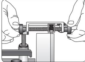
Check that the grinding wheel is exactly round and that the grinding surface is even. Adjust if necessary with the Tormek Truing Tool TT-50.
