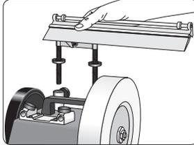
Remove the Universal Support and place the support in the sleeves of the machine. If required, remove the honing wheel.
