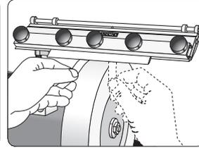
Make sure that the blade makes contact along the whole width of the wheel – a thin piece of paper simplifies this check. Adjust if necessary with the wheels (6).
