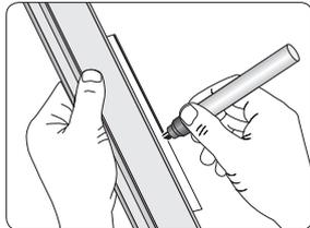
Colour the grinding bevel with a marker pen so that you can see where the grinding occurs when setting the edge angle.
