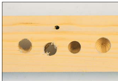
A 'new' bit cut the holes on the left, and a sharpened one those on the right
