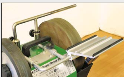
Slide the base plate onto the support, as far to the left as possible. Lock it in place temporarily
