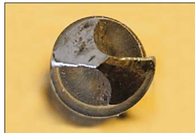
This close-up shows a standard twist drill bit in need of reshaping
