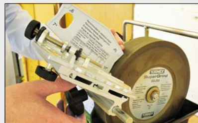
Tilt the base up and set it to the required clearance angle using the template
