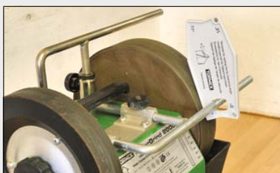
Set the universal support 14mm from the wheel using the hole in the setting template
