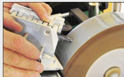
I found it best to give the nut 1½ turns, grind both sides and gradually adjust the stop nut to sneak up on the primary facet
