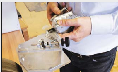
Mount the drill bit into the holder and set the length to the stop on the guide
