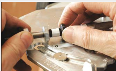
To cut the secondary facet, tilt the base away from the stone and move the drill holder forward up to the second mark on the guide. Then tilt the base forward until the point of the drill touches the stone. Adjust the stop nut to give the required secondary facet
