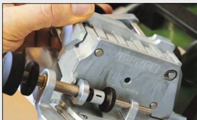
Place the drill holder on the guide and adjust the setting screw so the point of the bit just touches the stone. Then turn the setting screw inward to give the required cutting depth; one turn is 0.5mm. You can now cut the primary facet on both edges of the drill
