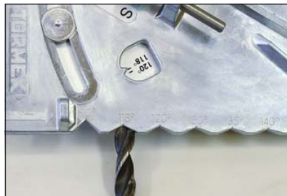
Check the bit's point angle by holding it against a groove on the edge of the guide
