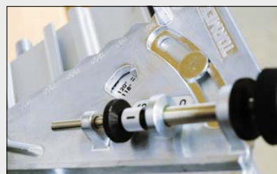
Set the point angle on the guide before sliding it onto the base plate
